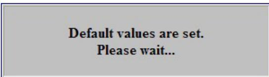
Affirming the query, all settings made on the EEPROM will be deleted and replaced by the default settings. The modul will go back to these default values. Once the setting process is over, there will be automatic return to the main menu.
