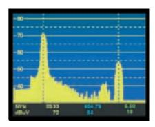
markers appear on the screen with indication of level and frequency gap between them. With 50 dB dynamic range, frequency or channel and level indication simultaneously on the screen the interpretation of the readings is immediate.
