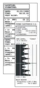
The results can be stored in the memory or also transferred to a printer to obtain reports right in the place where the measurements are made. For this purpose the CI-023 printer can be attached to the instrument's carrying bag.
